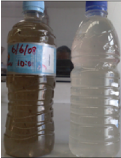
Wastewater from raw water pit and after biological treatment.
